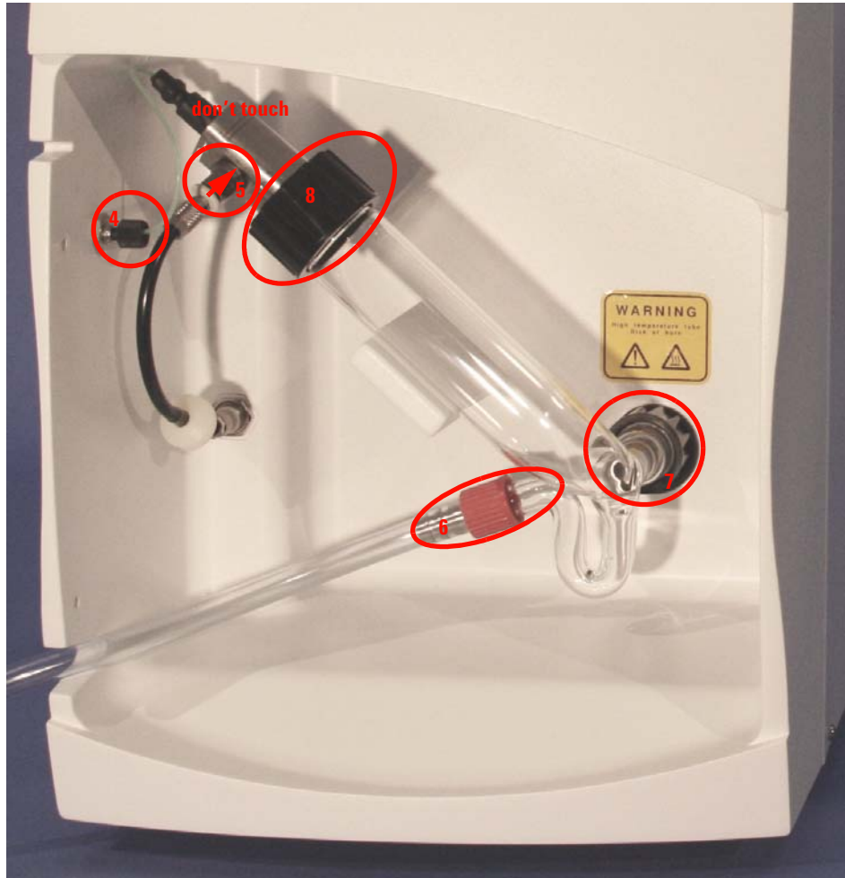
Figure 17 Replacing the nebulization chamber
