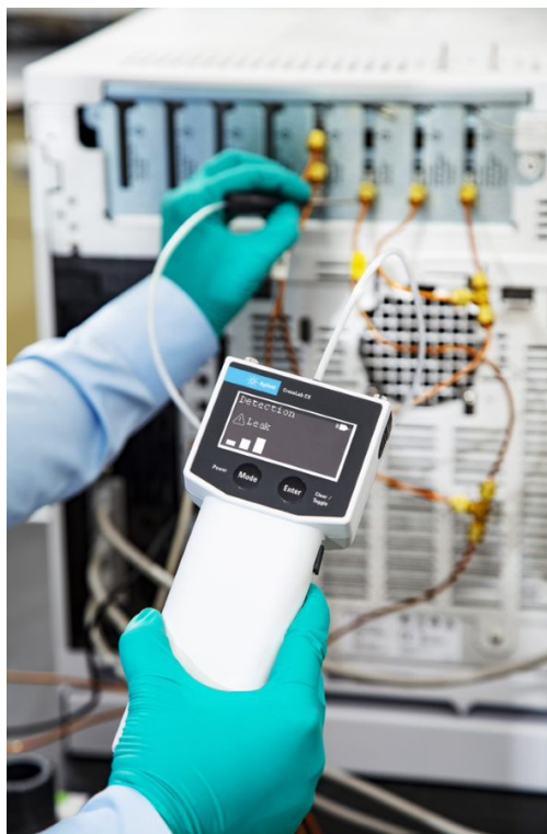
Figure 9. Example of leak checking gas fittings on the back of an Agilent 8890 GC.
