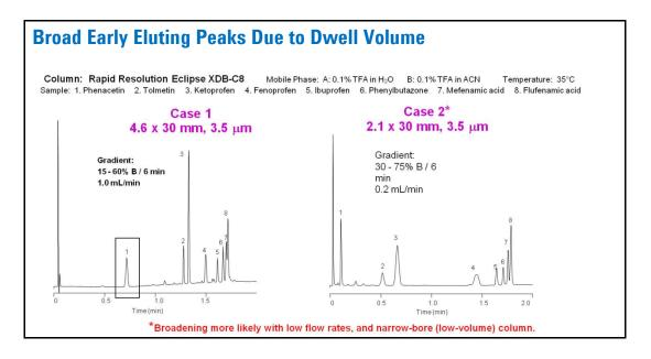
Knowing the dwell volume is important when transferring gradient methods to other instruments and laboratories.
