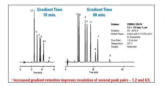
The longer gradient time results in a shallower gradient. By decreasing the gradient steepness, we're able to separate peaks 1 and 2, and 6 and 7.
