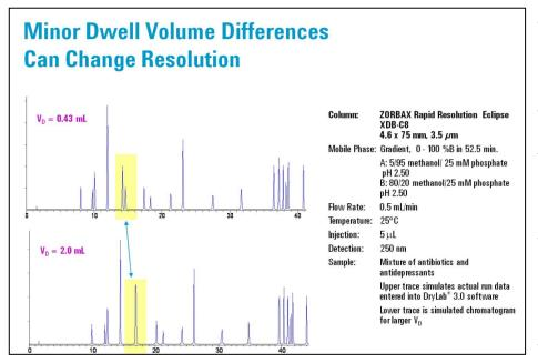
The example on the left represents simulated gradient chromatograms for separations of a complex mixture. The upper trace is a simulation of the actual input data. The lower trace is a simulated chromatogram of the same separation carried out on an instrument having a dwell volume of 2.0 mL instead of 0.43 mL. Notice the peak pair that separated on one instrument completely co-eluted on the instrument with the larger dwell volume.
