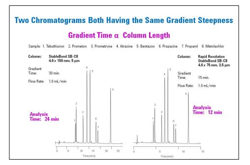
See the example above. In the chromatogram on the left, our sample is well separated on a 4.6 x 150 mm, 5um column using a gradient time of 30 minutes at 1.0 mL/min. We achieved a significant reduction in analysis time by reducing the column length to 75 mm. The gradient steepness was unchanged but the analysis time *decreased by 50%*. A reduction in solvent consumption and re-equilibration time was also achieved.
