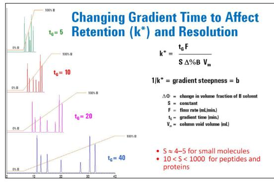
When gradient steepness is decreased, retention increases; when gradient steepness is increased, retention decreases.
