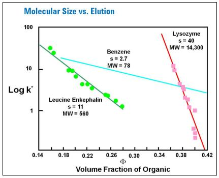
Different analytes have characteristic S values which reflect a molecule's sensitivity to the % organic in the mobile phase. See the example at the left.
