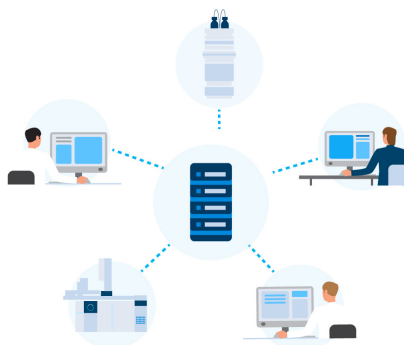
Figure 1. The client-server model interconnects workstations, instruments, and other devices to allow for centralized management, increased communication and collaboration, and improved productivity and cost-efficiency across the lab.
