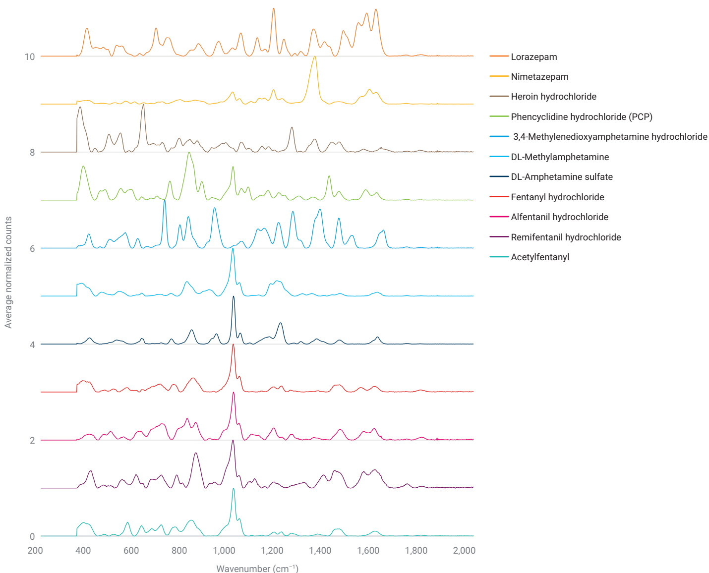
Figure 4. Averaged normalized spectra of the 11 narcotic certified standards used to build the SERS Narcotics library.
