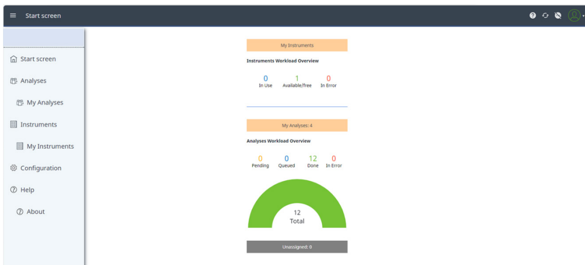
Figure 2. Start screen of the Agilent Sample Scheduler for OpenLab. Direct access to the respective information is available by clicking the boxes, graphics, and numbers. The menu on the left side can also be used for navigation.
