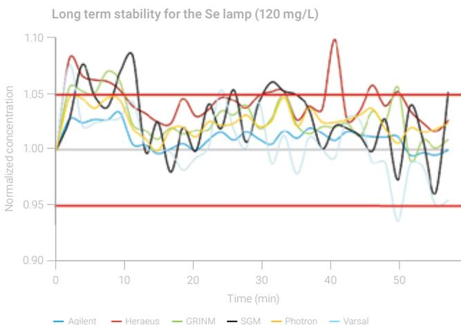
**Figure 14.** Long-term stability for selenium (Se) lamps based on measured absorbance for a 120 mg/L calibration standard. The solid red lines show control limits of  $\pm 5\%$  variation from the expected result. The Agilent lamp shows the best stability. The average precision for the Agilent lamp was  $<1\%$  RSD for all measurements over this 1 hour period, compared with the worst result of  $<3\%$  RSD for the Varsal lamp.
