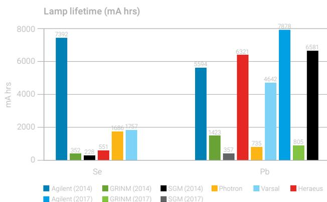
**Figure 16.** Lifetime of the selenium (Se) and lead (Pb) lamps. The Agilent lamp gave the longest life for both elements, well over 4 times longer than the nearest competitor for the Se lamp, and around 20% longer than the nearest competitor for the Pb lamp. The Agilent lead lamp tested in 2017 has an improved cathode composition, which improves both lifetime and performance compared with the lamp tested in 2014.
