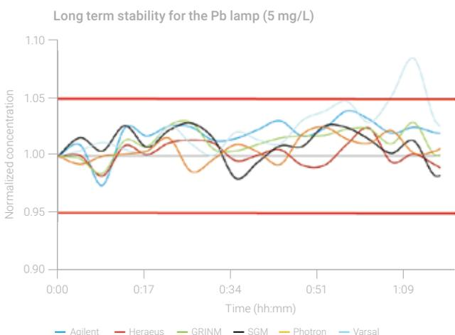
**Figure 15.** Long-term stability for lead (Pb) lamps based on measured absorbance for a 5mg/L calibration standard. The solid red lines show control limits of  $\pm 5\%$  variation from the expected result. The Agilent lamp shows good stability with an average precision of  $<1.6\%$  RSD for all measurements over this 1 hour period, compared with the worst result of  $>2\%$  RSD for the Varsal lamp.
