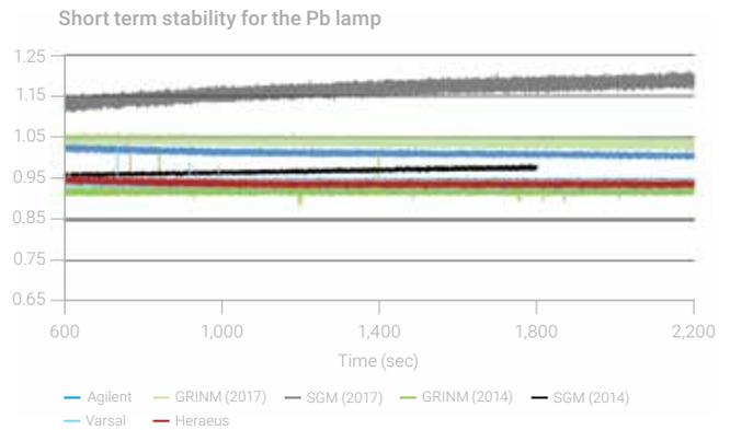
**Figure 13.** Short-term stability for lead (Pb) lamps, after a 10-minute warm up. While the Agilent and Heraeus lamps were suitably stable, the signals for both the Varsal and the GRINM lamps showed large spikes. The SGM lamps never appeared to stabilize.
