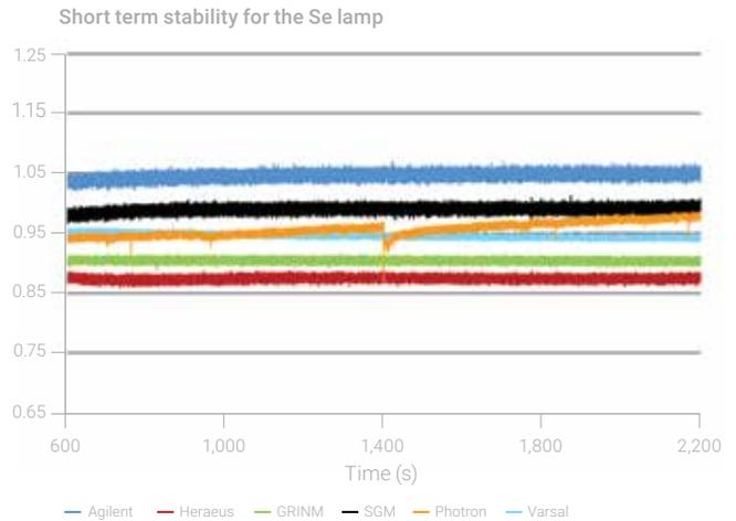
**Figure 12.** Short-term stability for selenium (Se) lamps, after a 10-minute warm up. While most lamps were suitably stable, the signal for the Photron lamp showed large spikes and never appeared to stabilize.
