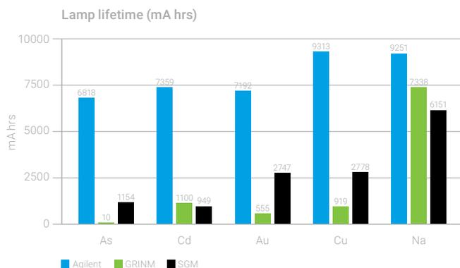
**Figure 17.** Lifetime for the arsenic (As), cadmium (Cd), gold (Au), copper (Cu) and sodium (Na) lamps. The Agilent lamp gave the longest life for each of these elements, well over 2.5 times longer than the nearest competitor for most elements, and  $>25\%$  longer than the nearest competitor for the sodium lamp.
