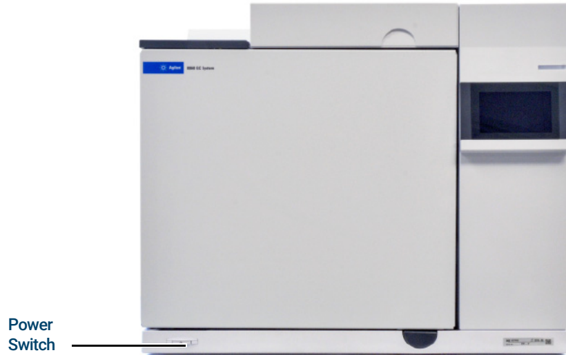
Figure 6. Power switch location
