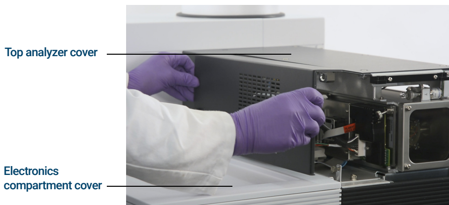
Figure 31. Installing the analyzer cover
