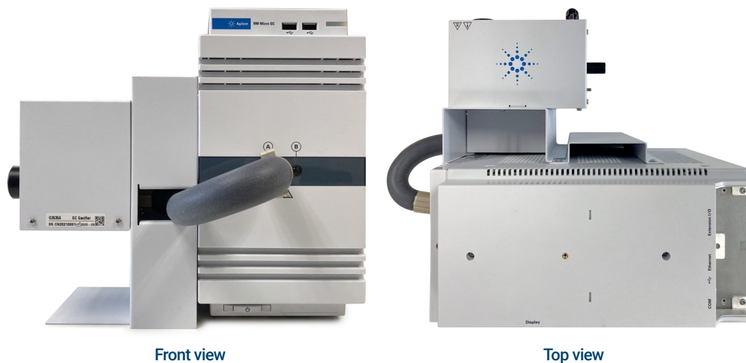
Figure 6. Transfer line connected to the 990 Micro GC.
