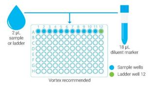
Femto Pulse system; Ladder – well 12, depending on which row is chosen
