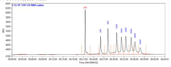
Representative Ultra Sensitivity RNA Ladder result, using the Femto Pulse System with the FP-1201-US RNA Kit. Peaks are annotated by size (nt). Method: FP-1201T22 -US Total RNA.
