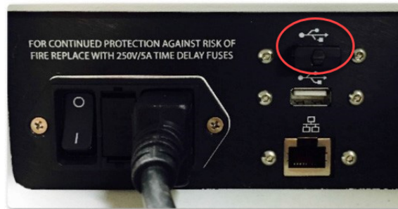
Figure 5. USB WiFi adapter inserted into an available USB port on the back of the XF HS Mini Analyzer
