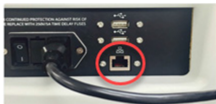
Figure 3. Ethernet (RJ-45) jack location outlined in red
