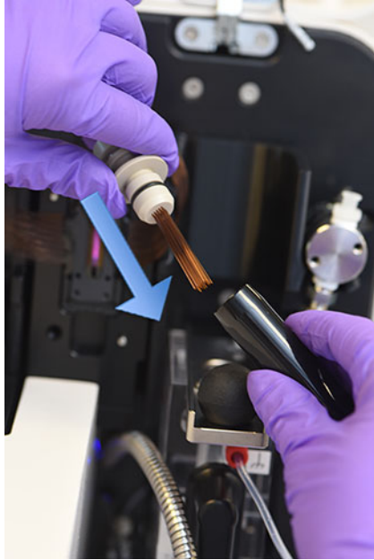
Figure 62 Instrument top compartment – installing protective cover
