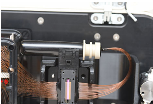
Figure 63 Instrument top compartment – storing covered capillary array bundle
