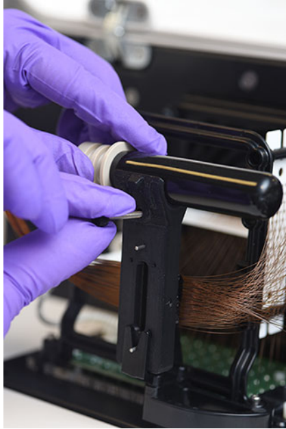
Figure 76 Instrument top compartment – remove array window
