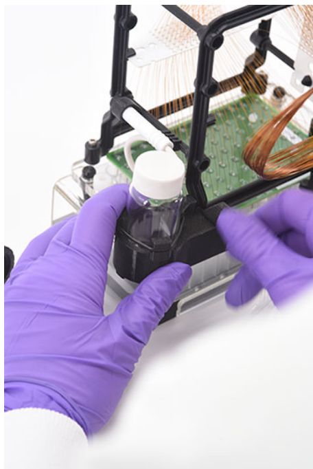
Figure 90 Array spindle storage device installation
