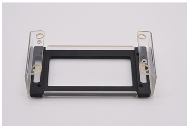
Figure 86 Array docking station with tray base installed
