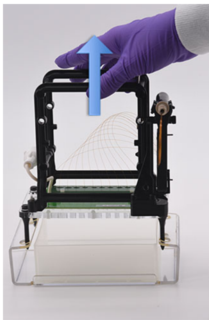
Figure 72 Removal of array from shipment frame
