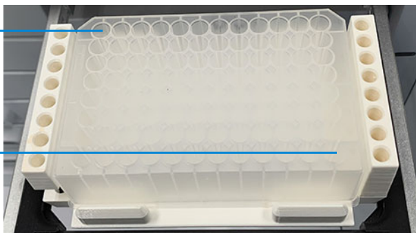
Figure 8 Proper orientation when loading 96-well marker and sample plates
