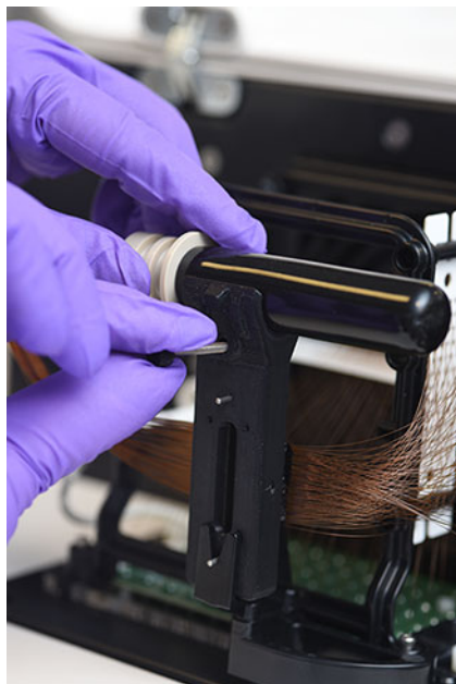
Figure 65 Instrument top compartment – attach array window to capillary array frame
