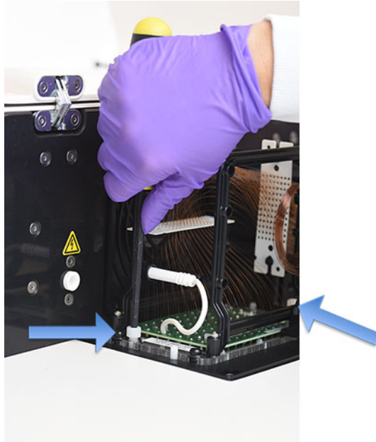
Figure 66 Instrument top compartment – array attachment screw removal
