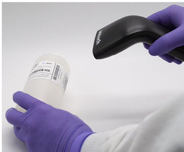
Figure 103 Scanning the bar-code of the gel
