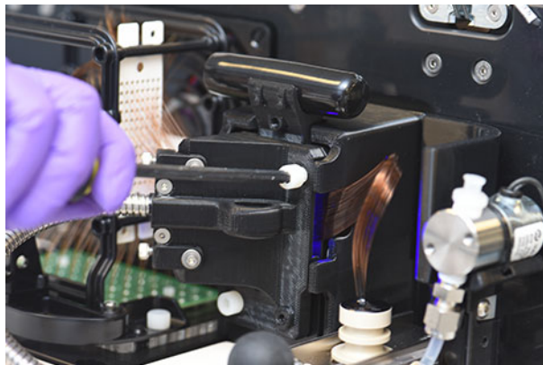
Figure 82 Instrument top compartment – light guide placement
