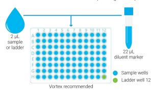
5200 system; Ladder – 12 capillary: well 12, depending on which row is chosen
