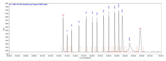
High Sensitivity Extended Large Fragment DNA Ladder result, using the Fragment Analyzer system with the DNF-464 High Sensitivity Large Fragment 50 kb kit. Peaks are annotated by size (bp). Method: DNF-464-33 (33cm "short" array).
