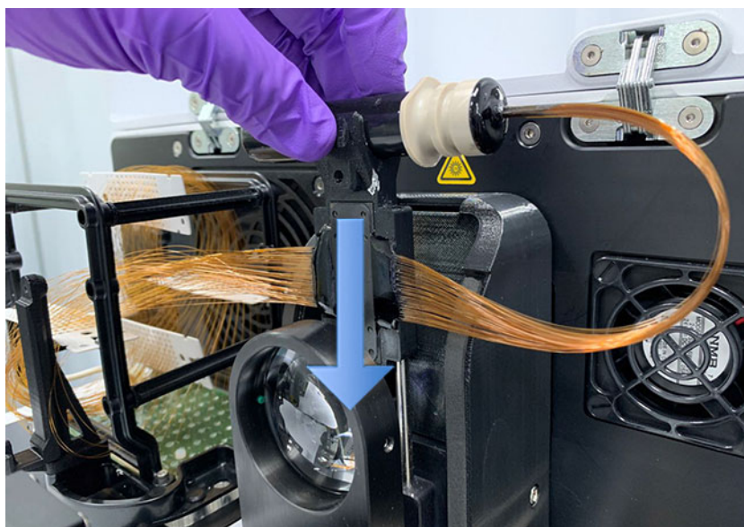
Figure 83 Instrument top compartment – array window placement
