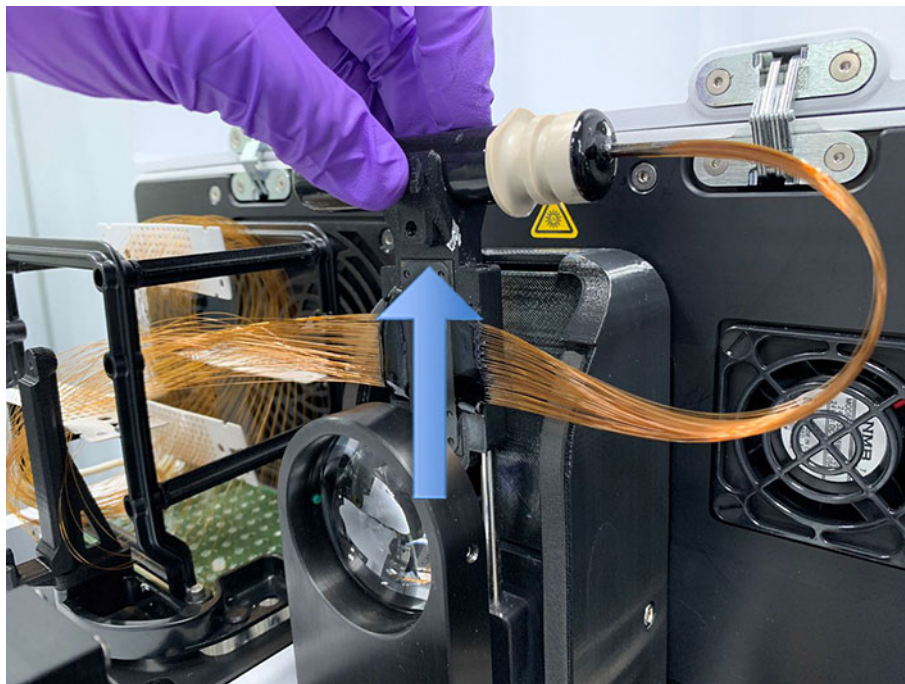
Figure 69 Instrument top compartment – remove capillary array window
