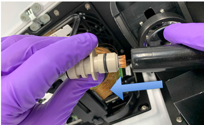
Figure 67 Instrument top compartment – installing protective cover
