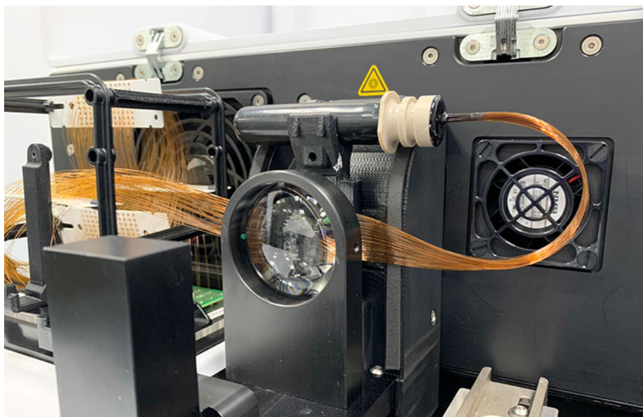
Figure 84 Instrument top compartment – capillary array bundle removal
