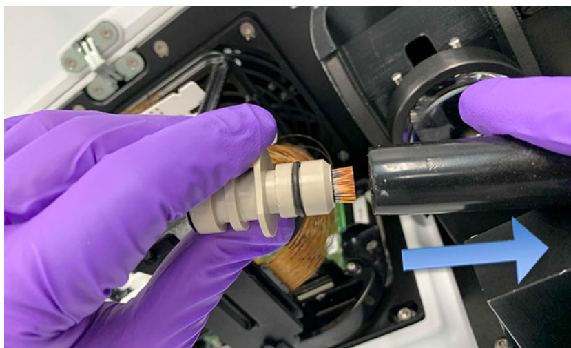
Figure 85 Instrument top compartment – removing protective cover
