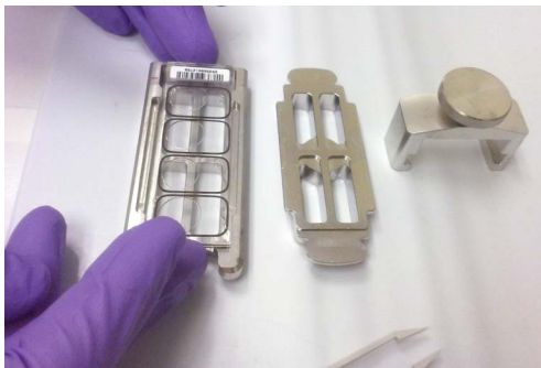
Figure 21 Removal of the microarray-gasket sandwich from the chamber base
