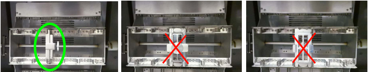
Figure 18 Assembled chambers in correct (left) and incorrect (middle and right) orientations
