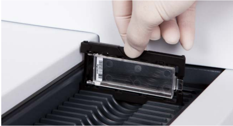
Figure 28 Inserting slide holder into cassette
