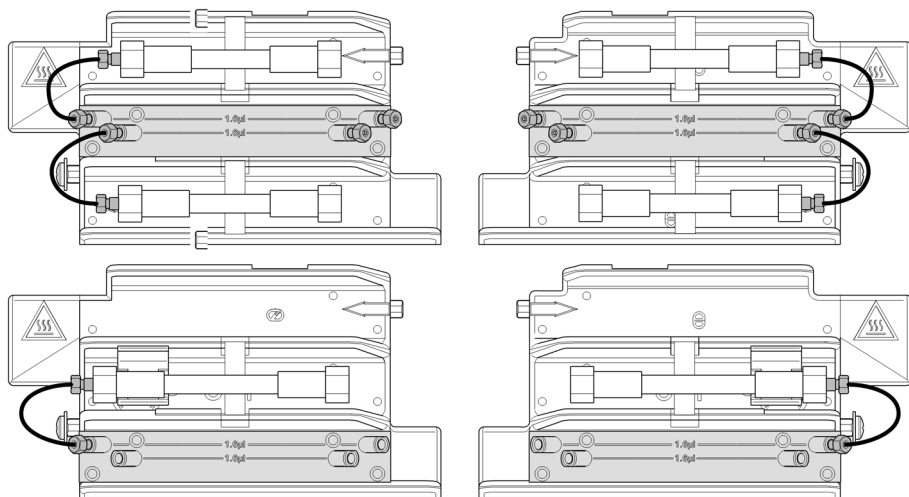
Figure 3 Arrangements of Heating and Cooling Devices (G1316C)
