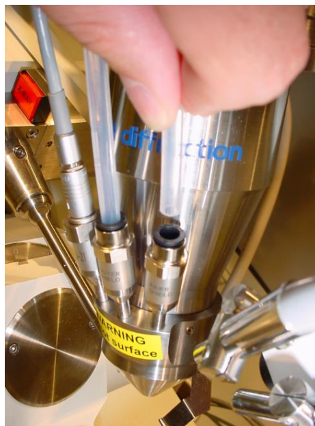
Figure 14 Attaching tubing to Helijet
