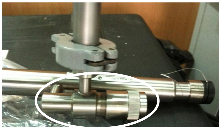
Figure 28 Vacuum pumping the Helijet head
