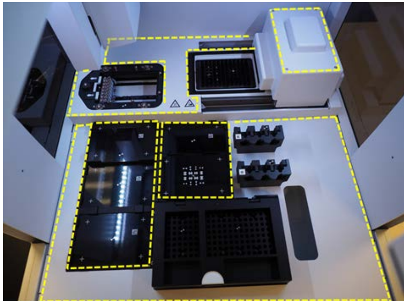
Figure 32 Deck surfaces to be wiped down
