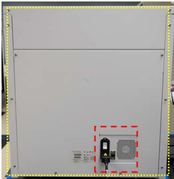
Figure 35 Exterior surfaces on the back of the instrument to be wiped down
