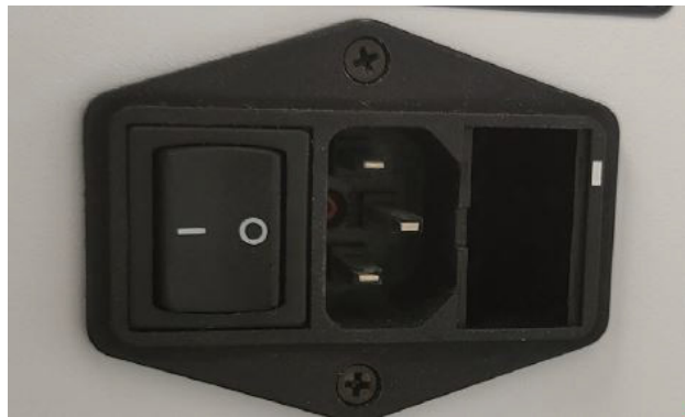
Figure 4. Power inlet module without fuse drawer, at the rear of the device.
