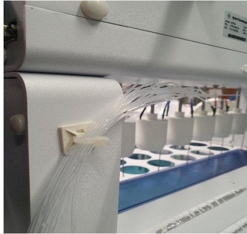
Figure 8. Rear View of the Bio-Disk with Self Adhesive Pad and Cable-Tie Applied
