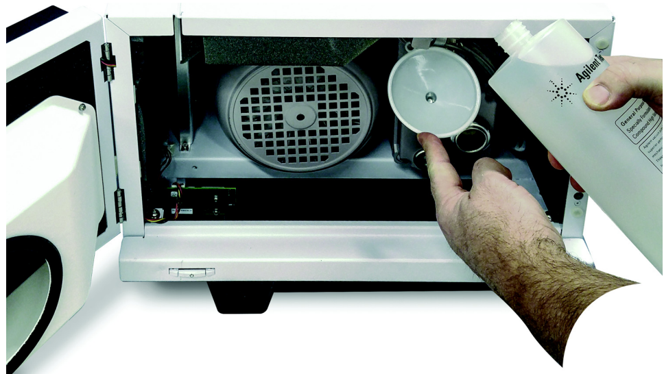
Figure 13. Refilling the pump with oil
