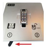
8. In one smooth motion, move lever to pos 1 to retract the slide rests.
