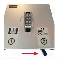
5. Move lever to pos 2 to prepare the slide rests for slide placement.
