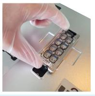
7. Place the microarray slide onto the slide rests (numeric barcode up).
