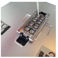
6. Load the samples into the gasket wells.
