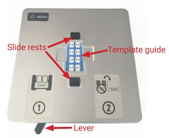
**Lever**: In the image, the Hyb Station is oriented with the lever on the bottom, but it can be used in any orientation that is ergonomically comfortable for the user. When the lever is in position 1 (as shown) the slide rests are retracted. Moving the lever to position 2 moves the slide rests slightly inward, preparing them for slide placement.
