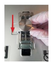
10. Slip on clamp. Slide until it stops in the center of hyb chamber.
