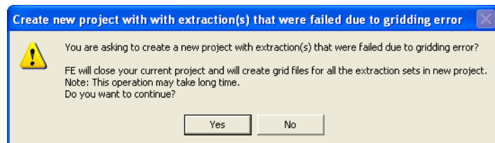
Figure 31 Failed extractions due to gridding error
