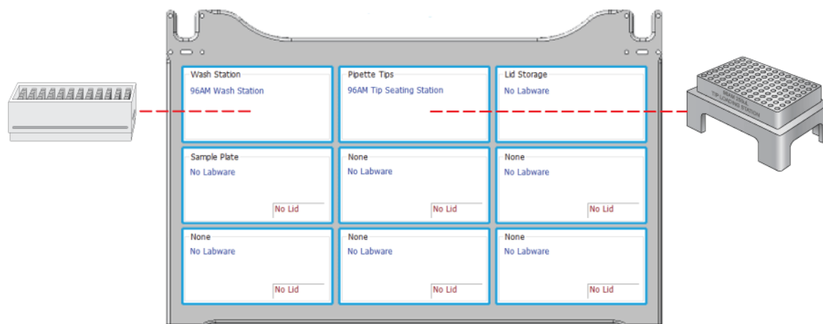
Figure Labware locations on the Bravo deck (top view)
