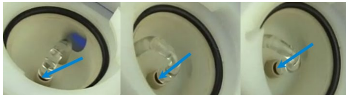
Figure 66. Even gap of around 0.5mm between the impact bead and the venturi throat
