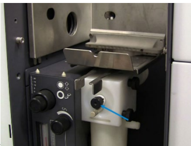
Figure 37. Thimble location. The locking ring is between the thimble and the nebulizer block
