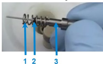
Figure 47. Insert spring over the capillary assembly 1. Spring 2. O-ring 3. Capillary assembly
