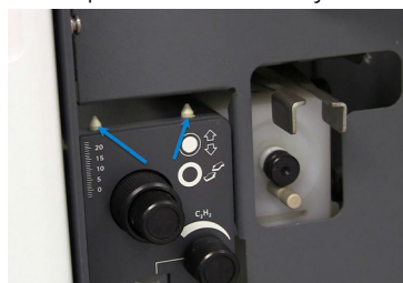
Figure 12. Lower Sample Compartment Front Panel over the two lugs on top of the burner adjuster.
