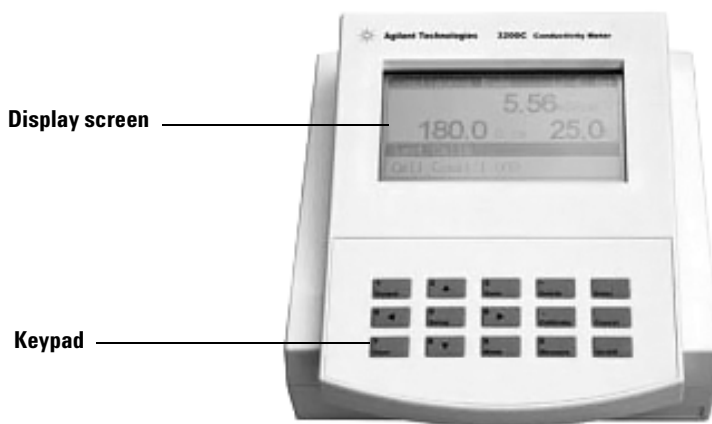
Figure 6 The front view of the 3200C Conductivity Meter
