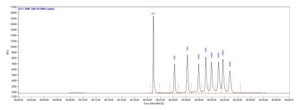
Representative HS RNA Ladder result using Fragment Analyzer system with the DNF-472 HS RNA kit (15 nt). Method: **DNF-472T33**. Peaks annotated by size (nt).
