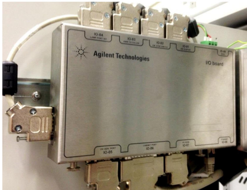
Figure 6 Safety IO Device
