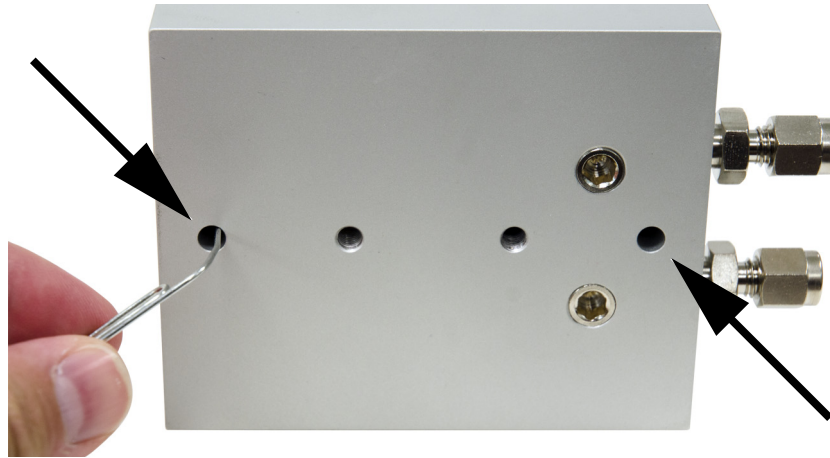
Figure 2. Removing the plastic caps from the connecting unit
