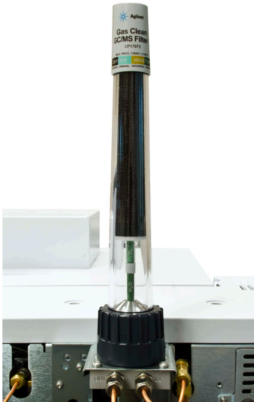
Figure 35. Carrier Gas filter installed to the bracket connecting unit, 7890 shown
