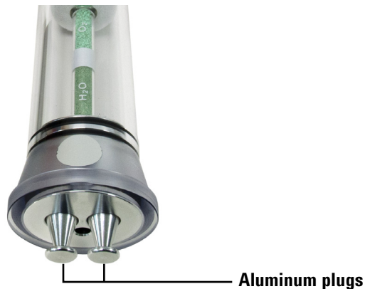
Figure 27. Remove the aluminum plugs from the filter
