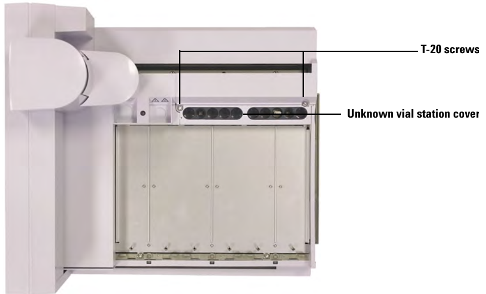
Figure 78 Removing screws and unknown vial station cover
