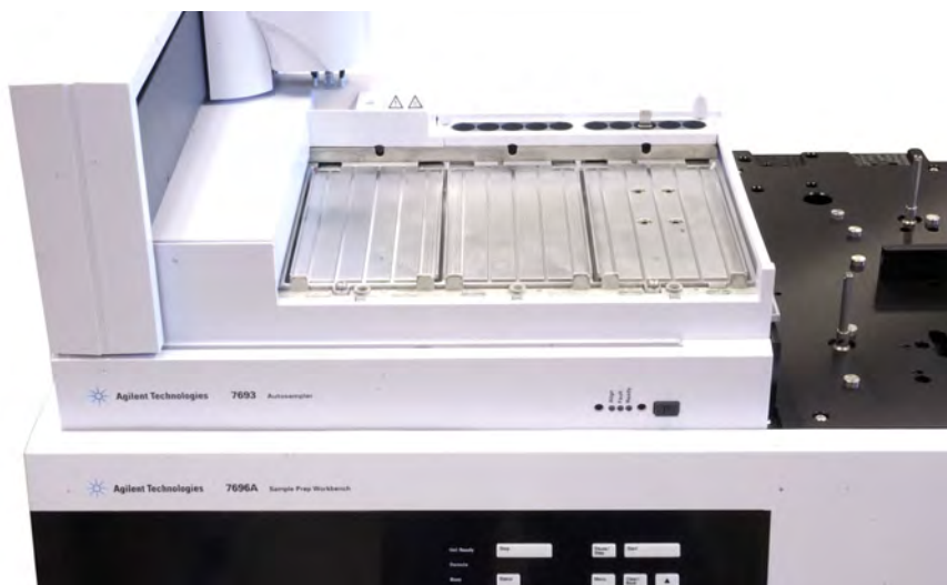
Figure 94 Sample tray with Peltier module sitting evenly on the main frame surface
