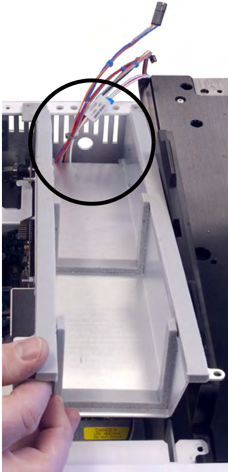
Figure 72 Installing the Peltier power control board bracket
