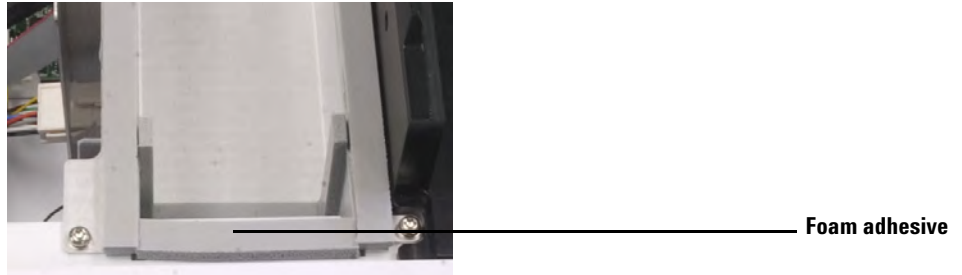
Figure 74 Installing the foam adhesive to the main frame chassis
