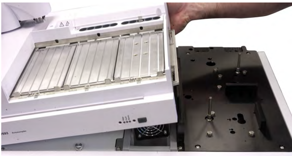
Figure 93 Lowering the sample tray onto the main frame chassis
