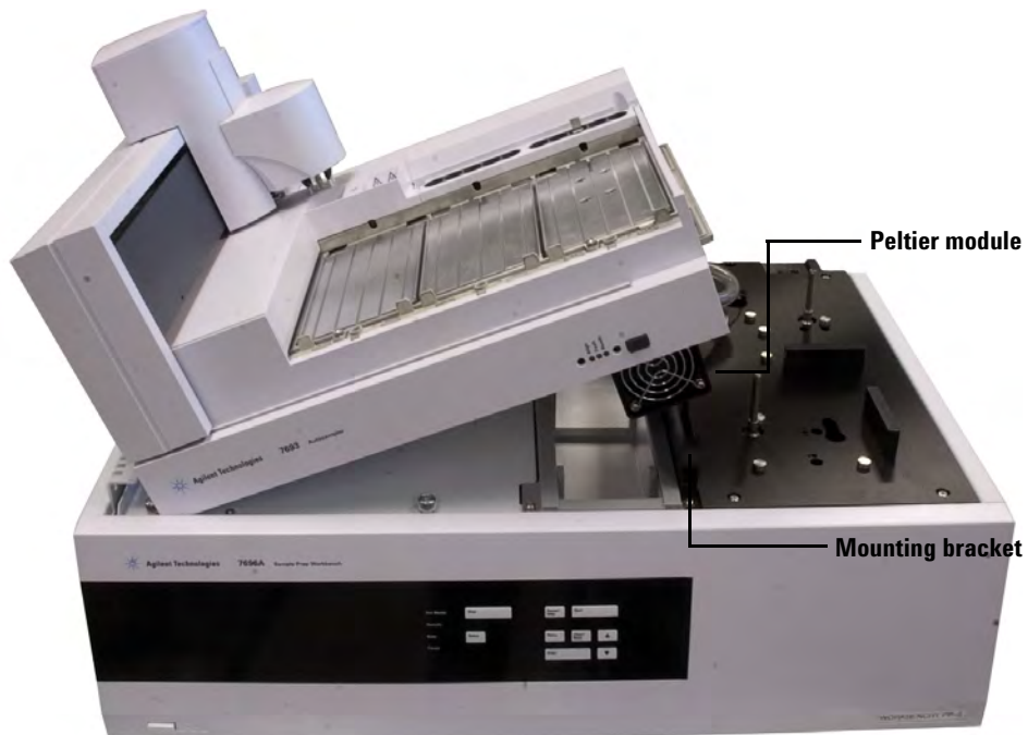
Figure 91 Propping the sample tray on the main frame with the Peltier module sitting on the mounting bracket
