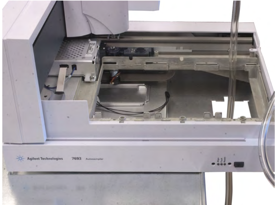
Figure 83 Running the drainage tubing through the accessory opening
