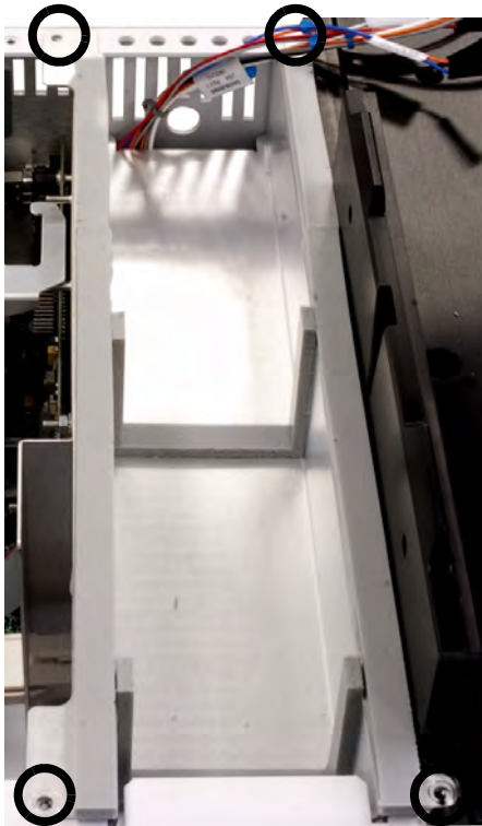
Figure 73 Installing the screws to the Peltier power control board bracket
