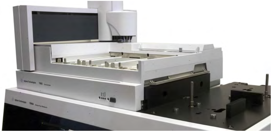
Figure 13 Setting the Sample Tray flat on the Main Frame base
