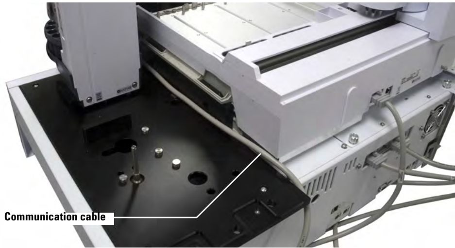
Figure 21 Running the front Tower cable along the Sample Tray mounting bracket.
