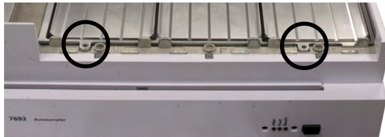
Figure 87 Installing two T-20 Torx screws to secure the front of the Peltier module
