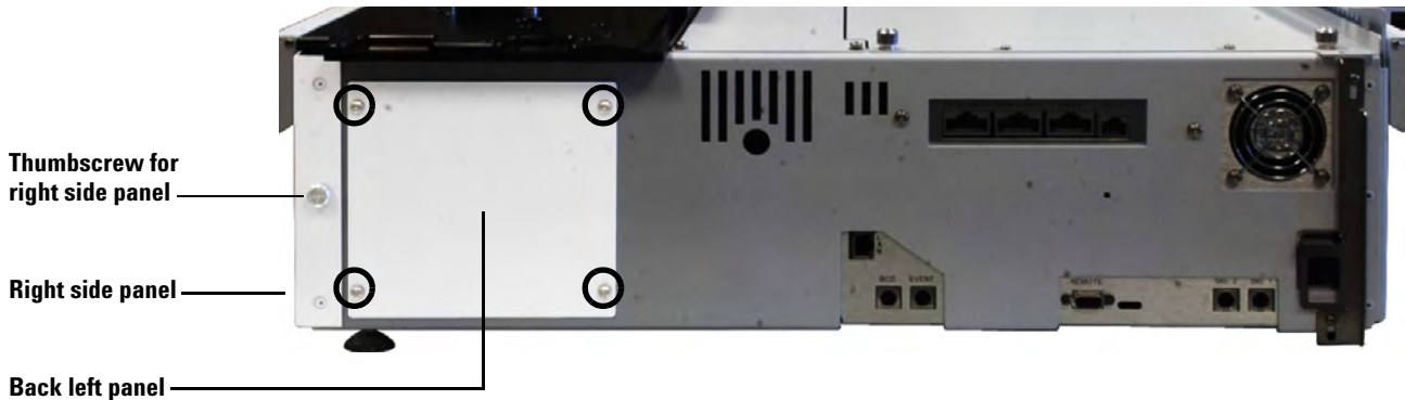
Figure 33 Removing the back left mainframe panel
