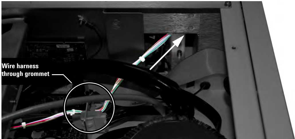
Figure 37 Wire harness run through grommet and mainframe chassis
