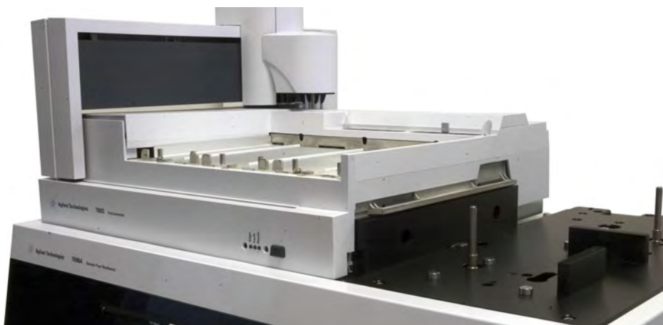
Figure 43 Setting the sample tray flat on the mainframe base
