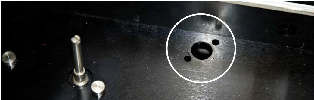
Figure 51 Align opening with knob on underside of weigh module
