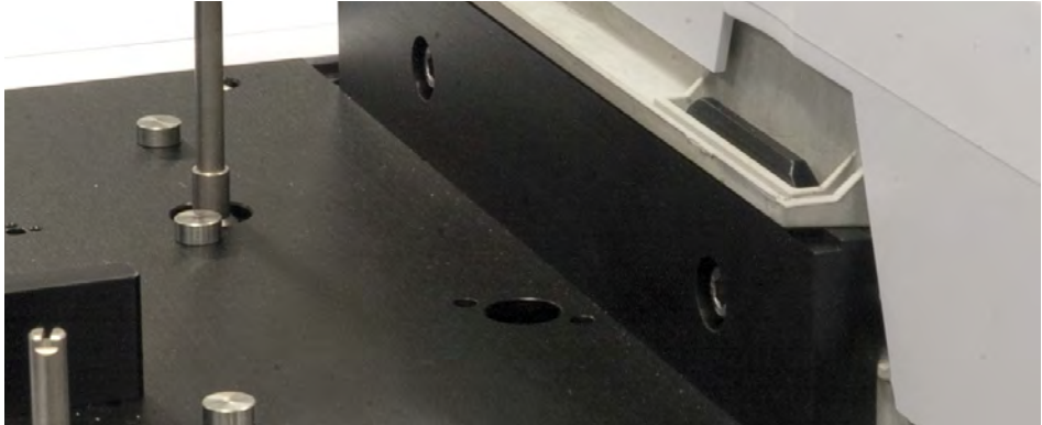
Figure 65 Removing the screws in the main frame mounting bracket
