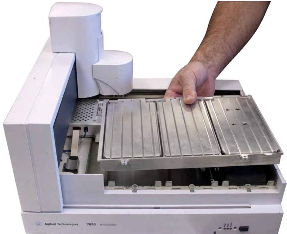
Figure 85 Installing the Peltier module
