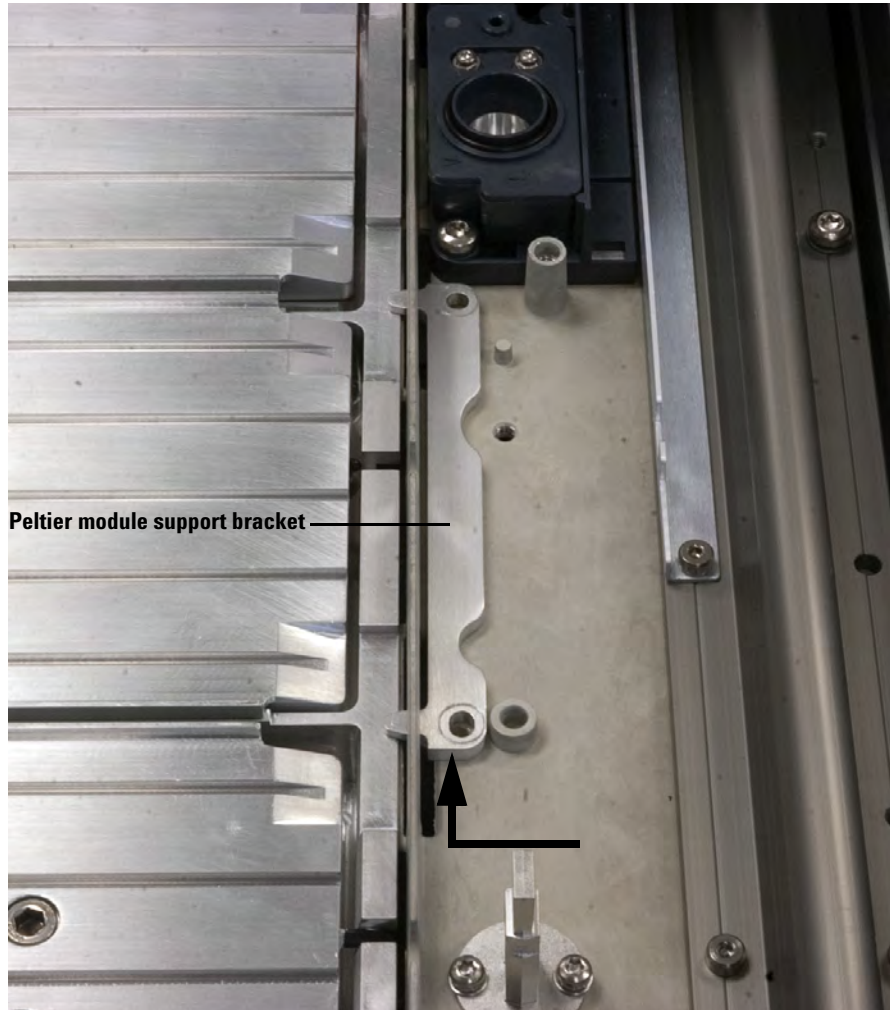
Figure 88 Installing the Peltier module support bracket
