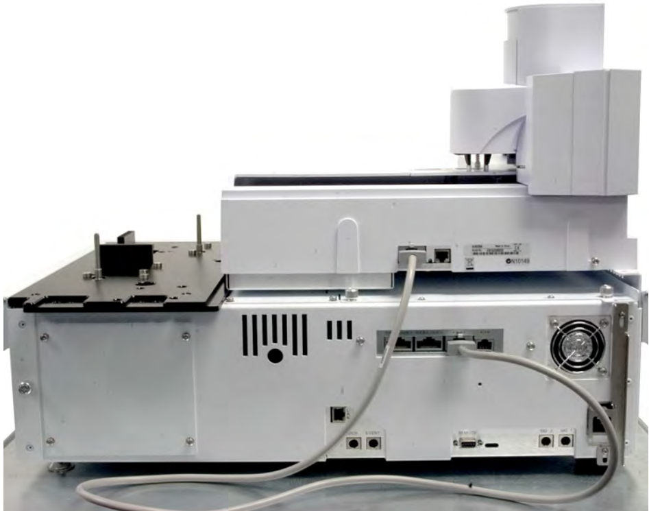
Figure 15 Connecting the Sample Tray communication cable
