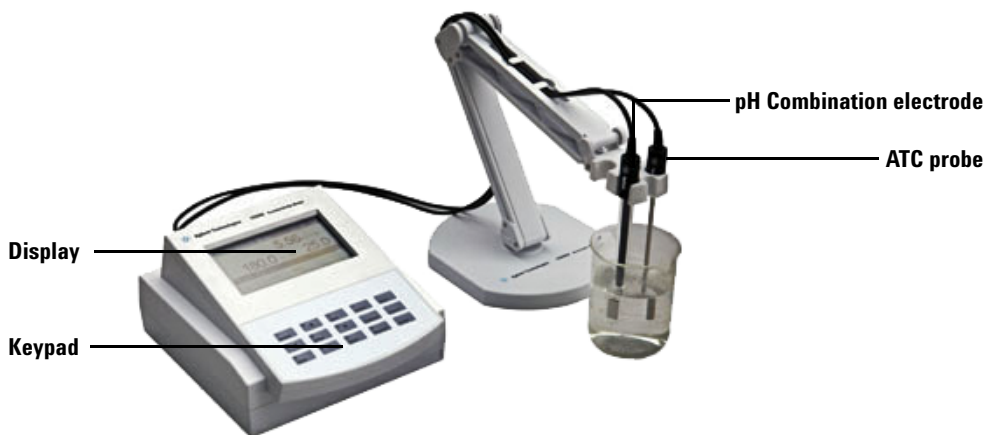
Figure 4 Major parts of the pH 3200P system
