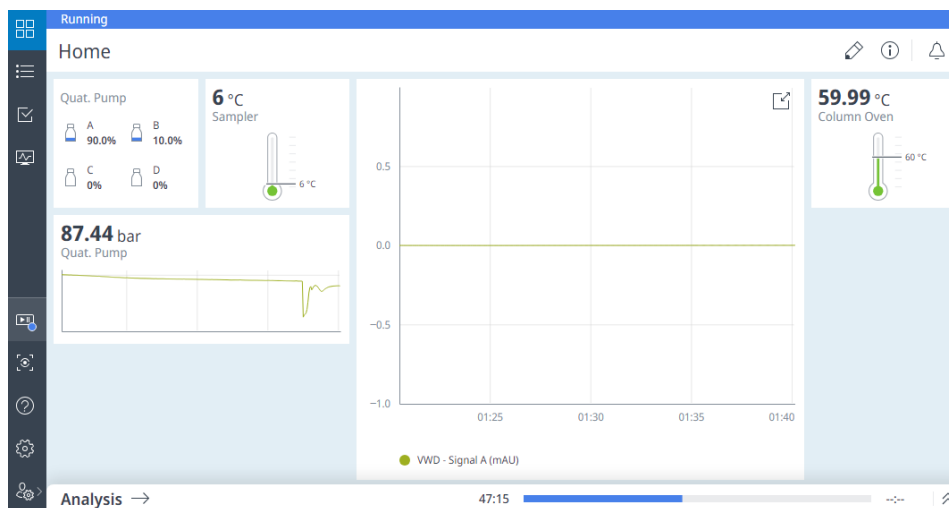
Figure 3. Home screen of the Agilent InfinityLab Assist, with the run control panel at the bottom showing that an analysis is in progress.
