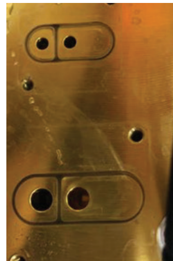
After 3.5 months use with genuine Agilent Cool Clear coolant, which includes corrosion inhibitor, the internal surfaces remain unblemished, confirming superior corrosion protection.
