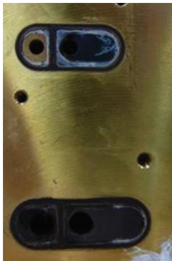
After 4 months use with de-ionized water, corrosion of the internal surfaces is easily identified by the darkened areas. The observed degradation is much worse compared to the use of non-genuine coolant.
