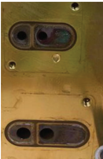
After 2 months use with non-genuine coolant, which does not include any corrosion inhibitor, corrosion of the internal surfaces is easily identified by the darkened areas.
