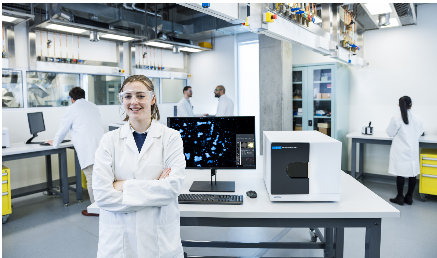
Figure 1. The Agilent 8700 LDIR chemical imaging system allows high-speed, routine analysis of microplastics, including the number of particles present in the sample, their size, and their chemical composition.
