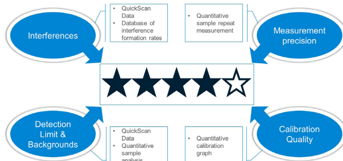
Figure 2. IntelliQuant star rating uses multivariate analysis to calculate a confidence level for the quantitative sample data
