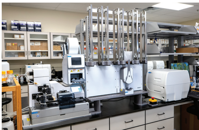
Figure 1. Agilent BioTek 406 FX washer dispenser, Agilent PlateLoc thermal microplate sealer, Agilent BenchCel microplate handler, and Agilent BioTek Cytation 7 cell imaging multimode reader.
