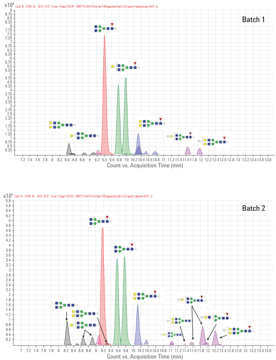
Figure 4. Comparison of the glycan profiles of two monoclonal antibody production batches, analyzed using the mAb-Glyco Chip. Batch 2 has a higher percentage and greater variety of sialylated glycan forms.
