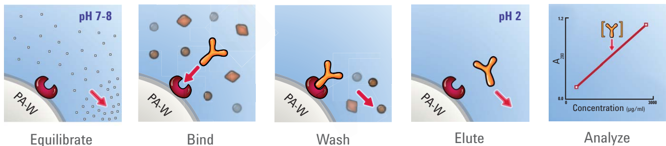
Figure 1. The complete capture workflow for the Agilent Bravo for Protein Purification system equipped with AssayMAP Protein A cartridges, as it would be used for protein titer analysis. Protein A captures the mAb at neutral pH; the mAb is then eluted at low pH using an acidic buffer. A calibration curve can be created to accurately measure the concentration of a mAb produced in a bioreactor.
