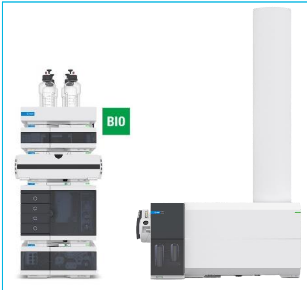
Figure 1. Standardized LC configuration used a 1290 Infinity II Bio LC (left) which is metal free to give best peak shape of metal sensitive analytes. Coupled to it is a Revident LC/Q-TOF (right) which provides robust and reliable small molecule analysis. Not shown is a Metabolomics Bravo platform for sample preparation.
