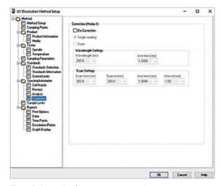
Figure 5. Correction for spectrometer section.
