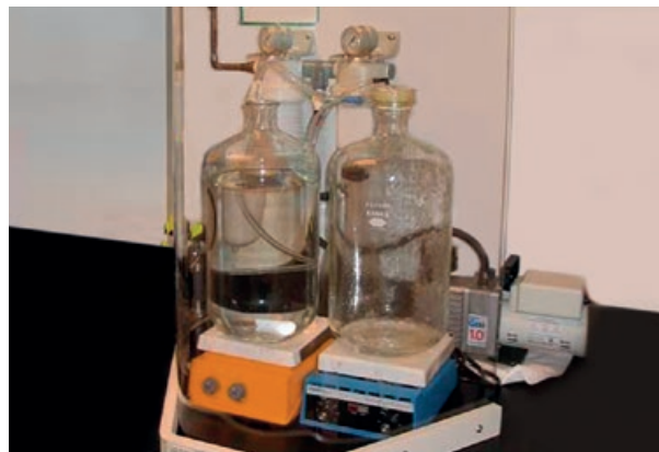
Figure 4. Typical laboratory deaeration setup according to the USP.
