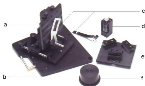
**Figure 1.** The Solid Sample Holder accessory.
