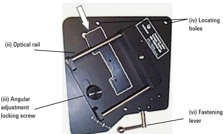
**Figure 3** showing (i) how to position the lower half of the clamp (outlined in white) under the optical rails (ii) on the accessory base. Locating holes (iv) and fastening lever (vi) are also labeled.
