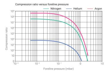
(\*) Measured with a 60 m³/h forepump.
