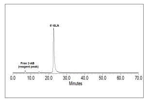
Figure 1 - HPLC results: 6'-SLN labeled according to the Signal<sup>™</sup> 2-AB Labeling Kit (GKK-404) and analyzed on a GlycoSep<sup>™</sup> N column (GKI-4728) in ammonium formate/acetonitrile.
