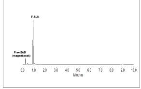
**Figure 3** - 6'-SLN labeled with 2-AB and analyzed on a Waters ACQUITY<sup>®</sup> UPLC<sup>®</sup> BEH Glycan column (1.7  $\mu$ m, 2.1 x 100 mm) in ammonium formate/acetonitrile.
