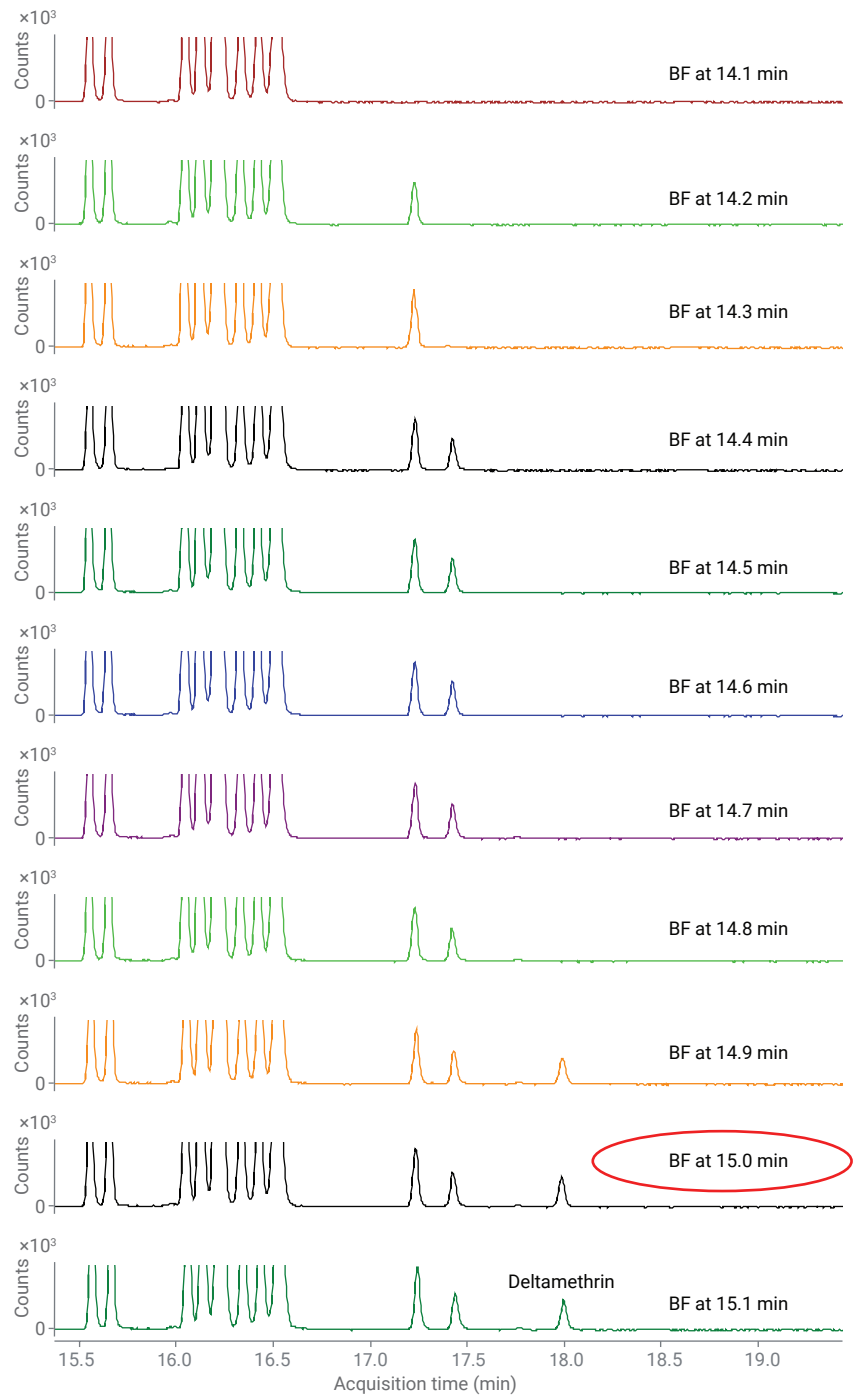
Figure 36. Optimization of the concurrent backflushing start by monitoring peak areas of late eluting analytes (especially the last analyte deltamethrin), thus their transfer from the first to the second column, at different backflushing (BF) start times (14.1–15.1 minutes).
