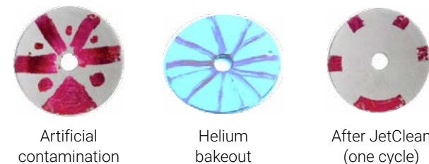
Image of ion lenses after helium bakeout and after one JetClean cycle.
