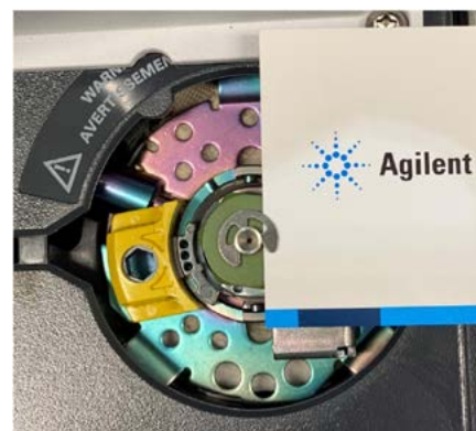
Proper height of a correctly installed septum nut.
