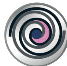
Gas exhausted at center hub
