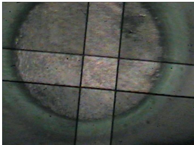
Figure 3. The visible image of Sample 2 including ViewThru apertures of the Agilent microscope. Analysis area is represented by the square box formed by the four aperture blades in the image center
