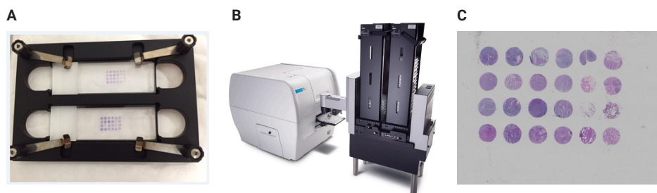
Figure 1. (A) Two TMA slides are positioned in a slide holder compatible with robotic interface to an Agilent BioTek multimode imaging reader (B). Software was preprogrammed to sequentially load each slide holder from the robot to the imager that then captured 15 \times 15 images of each slide using automatic montage and stitching features to illustrate the final array, shown here on one of the TMAs at 4 \times (C).
