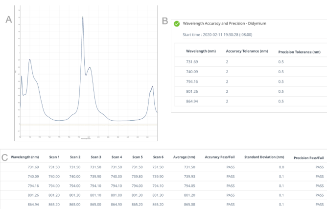
Figure 5. Wavelength accuracy test results for the didymium filter. (A) Six wavelength scans of didymium; (B) peak positions and tolerances; (C) raw peak positions for each individual scan tabulated along with the average, standard deviation and the pass/fail result.
