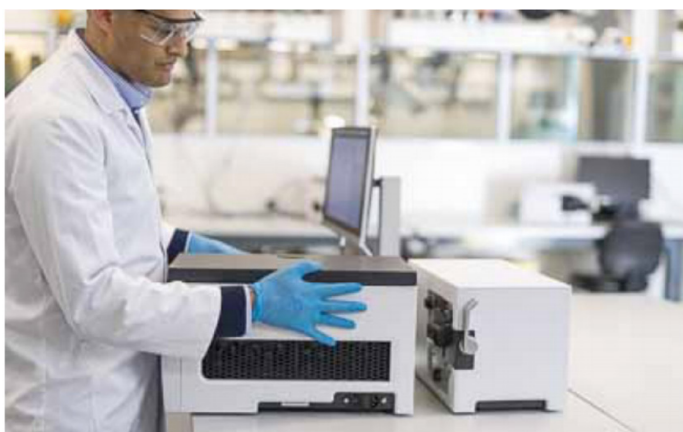
Figure 1. The Cary 3500 Multicell spectrophotometer consists of two parts: the engine (shown on the right) and the multicell module (on the left). The two parts are connected to create the complete spectrophotometer.
