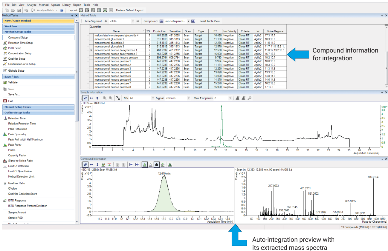
Figure 4A. Compounds from the PCDL were input into MassHunter quantitative analysis for an auto-integration method. Each compound was given a name, retention time, noise region, and m/z ratio(s). A representative spectrum was used to ensure that the software finds the correct peaks with the given parameters.
